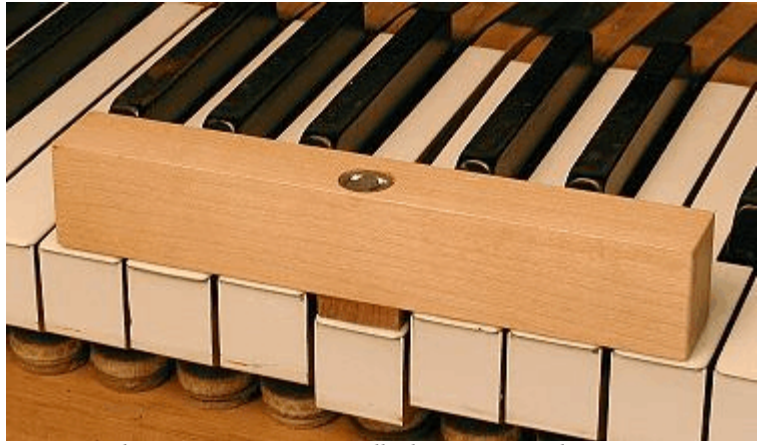
Figure 2: The ratio tester automatically depresses a test key 6mm
