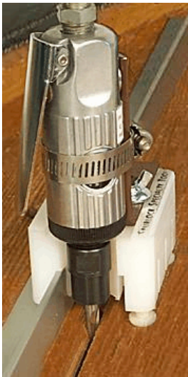
Routing parallel to fence
