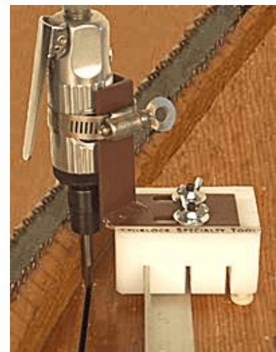
Bit extended, routing up to bridge
